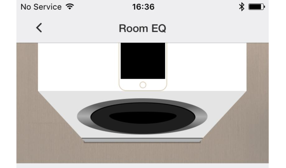
Place this device on top of the subwoofer with the bottom of it facing a side with a driver, as depicted above. Once you proceed, the subwoofer will emit a tone to use for calibration.
