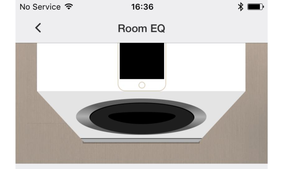
Place this device on top of the subwoofer with the bottom of it facing a side with a driver, as depicted above. Once you proceed, the subwoofer will emit a tone to use for calibration.
