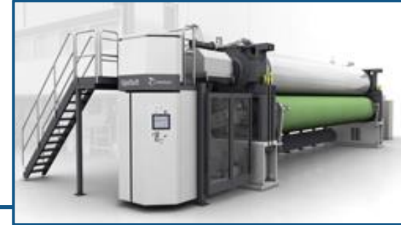
Metso's papermaking equipment. The machine's calender is controlled by a digital hydraulic system.
